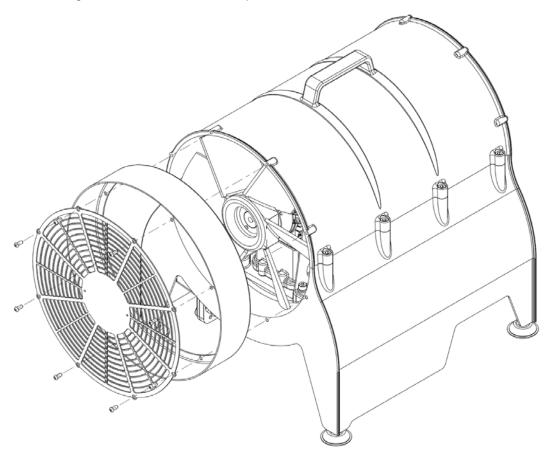
Fig. 1 Exploded diagram of fan guard and duct bracket
